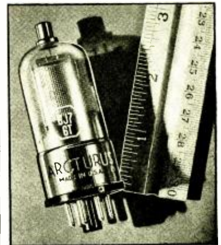
Designed for small sets, 7 new types of midget tubes have been engineered by Arcturus, & are available. Long used by mfrs., they are now going to jobbers & thence to dealers & public.
