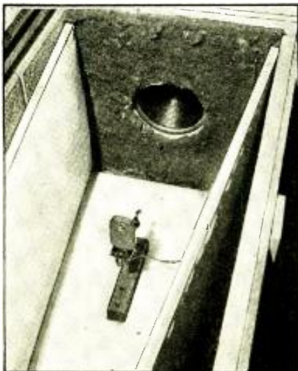
Fig. E. In a sound-proof chamber, test frequencies are picked up by the hear-aid mike.
