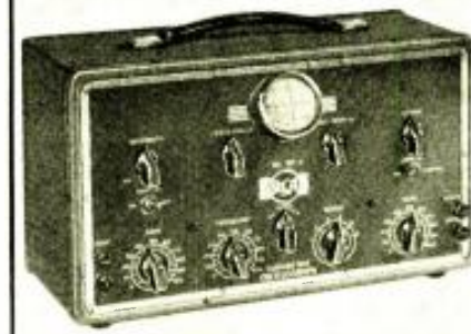
ABOVE, RCA 154 beat freq. oscillator has less than 5% distortion over entire range. BELOW, new 2-inch C-R Oscilloscope. Both are scheduled for early production; should be out by now.
