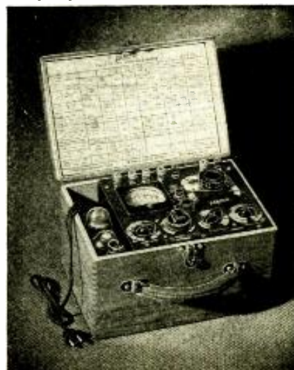
New condenser and resistor bridge. (1676)
